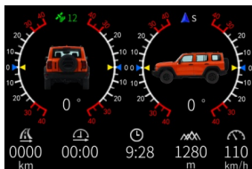
Off-road vehicle slope meter display
